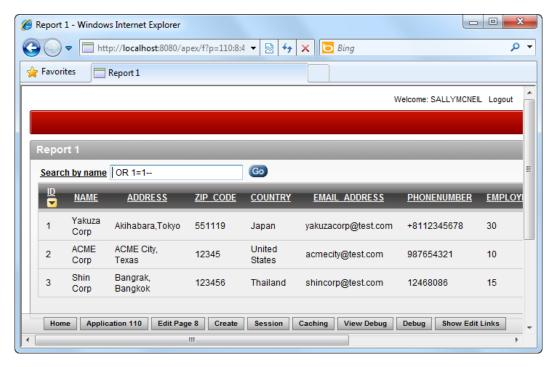
Figure 8-17. Conducting the SQL injection attack
