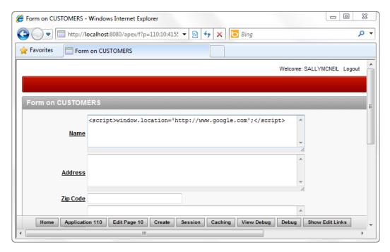
Figure 8-22. Conducting the cross-site scripting attack
