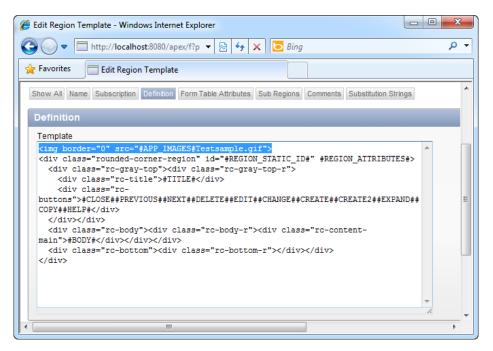
Figure 4-4. Including the Testsample.gif image in the template
