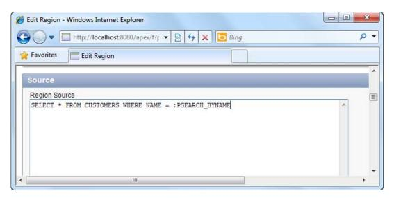
Figure 8-18. Using bind variables to protect against SQL injection attack
